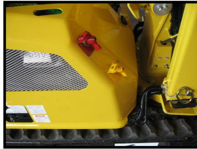
Battery & Starter Isolators
